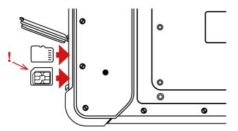
BE CAUTIOUS when inserting a SIM card or memory card and follow exactly the instructions in our manual. A card slipped upside down (be careful: the picture of the operating instructions shows the BACK SIDE of the tablet) or crooked may damage the contacts of the port. This is not covered by the guarantee. In addition, the port is a bit large and if you force the insertion of the card obliquely, it could slip inside the tablet.
